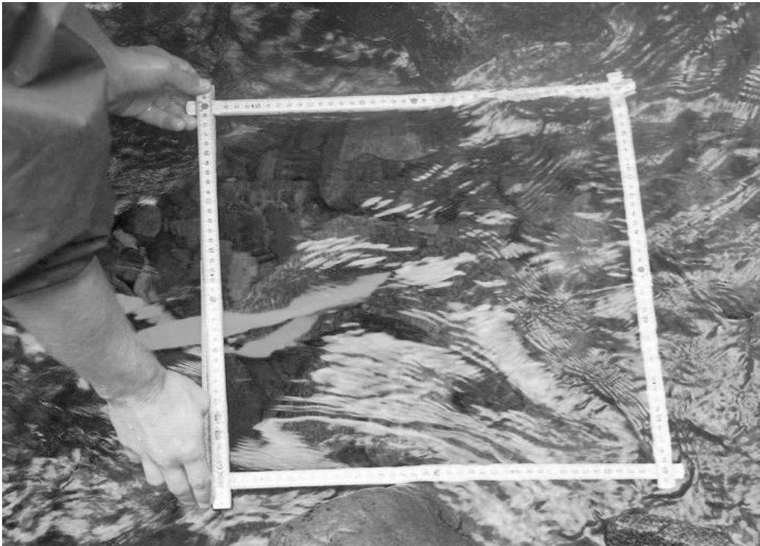
Figure S2. Fine-scale habitat assessment array used to measure percent cover of substrate sizes over the point of capture for A. truei larvae in northwestern British Columbia, Canada.
